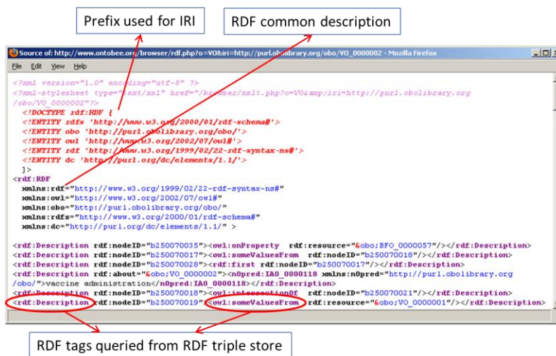
Fig. 3. Demonstration of an Ontobee RDF output file. This is also part of the source page view of the ontology term http://purl.obolibrary.org/obo/VO_0000002 (label: ‘vaccination’ from VO).
