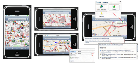
Fig. 16. Browsing through central London on DBPedia Mobile 58 ; we zoom in to an ROI and select a resource of interest. Representative icons distinguish resource types, e.g., hotels (using a bed) and music venues (musical notes). Overlaid on the snapshots are the UIs for forms-based querying and publishing new data to the LOD cloud.
