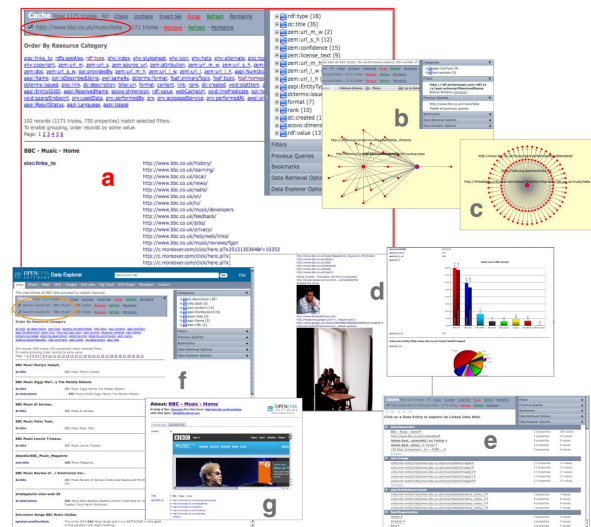
Fig. 20. The results are shown in ODE for a request for the URI http://www.bbc.co.uk/music/beta in (a); with alternative views – a filtered and the default RDF graphs in (b) and (c) respectively; two snapshots from the image view (d); and the navigator view in (e). The relationship to the query for the string “BBC Music” is shown bottom, left (f); and a new browsing chain is started in (g).
