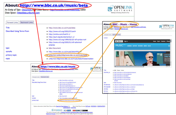
(a) Browsing from the resource URI for BBC Music Beta . On the right-hand side a template is used to display the result that includes the dereferenced URI (that retrieves the image) embedded in the output.
