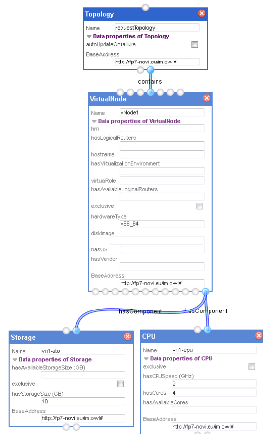
Fig. 6. Unbound request for one Virtual node with cpu/storage requirement
